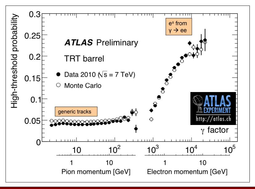
Transition radiation intensity proportional to particle relativistic factor  $\gamma$ =E/mc<sup>2</sup>. Onset for  $\gamma \sim 1000$  (MC tuned with test-beam data only)
