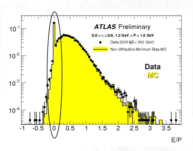
E/p measurement of 0 means **no calorimeter energy** assigned to a good isolated track...
