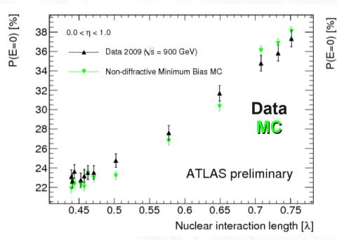
P (E=0) depends on the amount of material in front of the calorimeter
