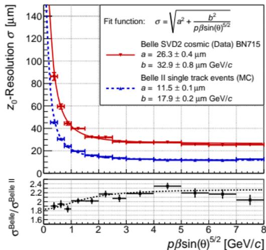
: Resolution of the transverse  $d_0$  (left) and longitudinal  $z_0$  (right) impact parameters. The results for MC events with a single muon track using the Belle II tracking algorithm are compared with the results for Belle cosmic events. The resolution in each bin is estimated using the  $\sigma$  value of a single Gaussian function fitted in a region containing 90% of the data around the mean value of the distributions.
