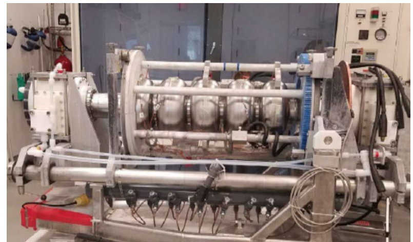
First 802 MHz cavity successfully built (Jlab)
