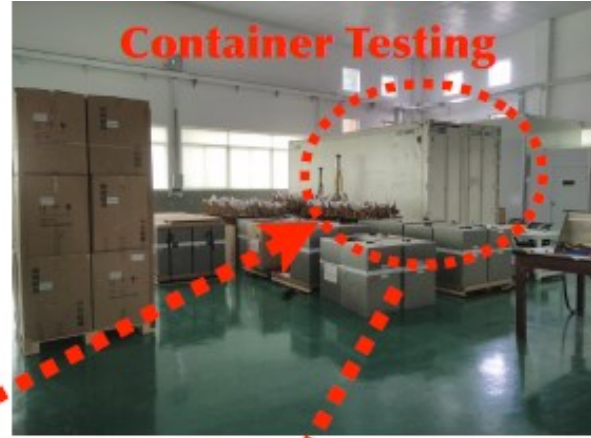
An Earth Magnetic Field (EMF) shielded 36-slot container testing all PMTs
