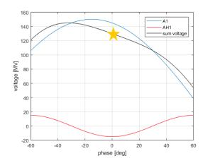
Tuning one of the Taylor coefficients do not change the others, especially the beam energy is not changed (provided that the oncrest phases are correct)
