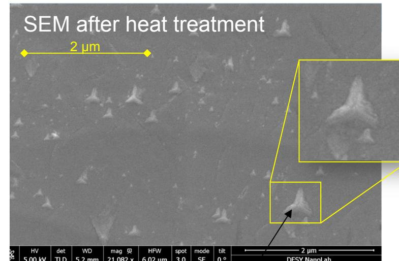
'star-like' precipitates identified as carbon using advanced surface analysis techniques
