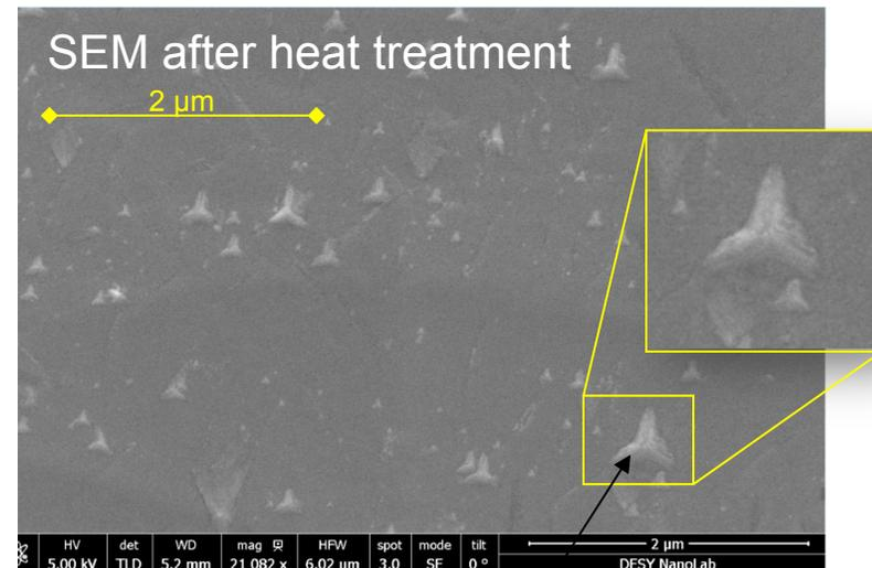
'star-like' precipitates identified as carbon using advanced surface analysis techniques
