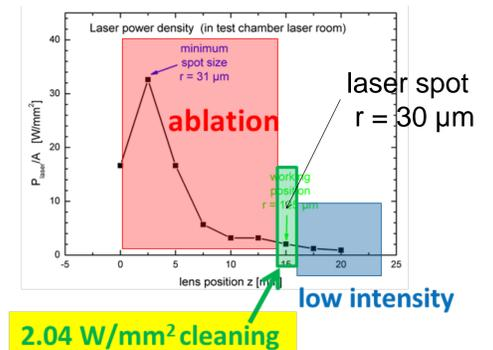
2.04 W/mm<sup>2</sup> cleaning (photoemission in gun 0.1 W/mm<sup>2</sup>)
