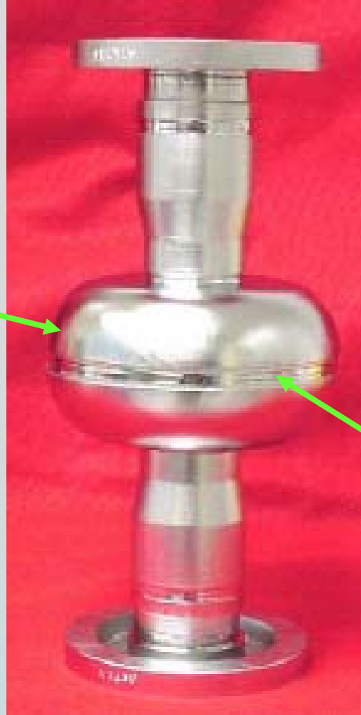
WELDED AREA: large grain size Machine marks (like grooves), large grains and height steps at GBs are well visible
