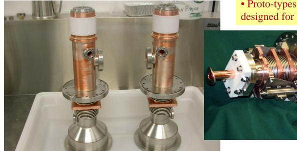
• Proto-types tested to 50 kWCW, 80 KW pulsed, designed for 75 kWCW
