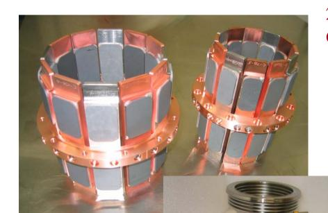
2 proto-types fab'ed by LEPP6 production loads fab'ed by ACCEL
