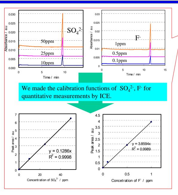
We could separate  $SO_4^{2-}$  and  $F^{-}$  in EP acid by ICE, and we also made the calibration functions of  $SO_4^{2-}$  and  $F^{-}$  for the quantitative measurements .
