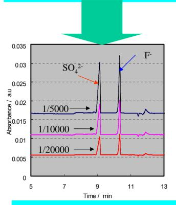
In this study, we performed the measurements of F- concentration in the EP acid with this calibration function.
