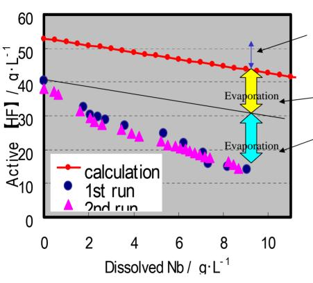
Finding 2 A half of Active **[HF]** escaped when dissolved Nb reached to 9 g/L at the end of EP process.
