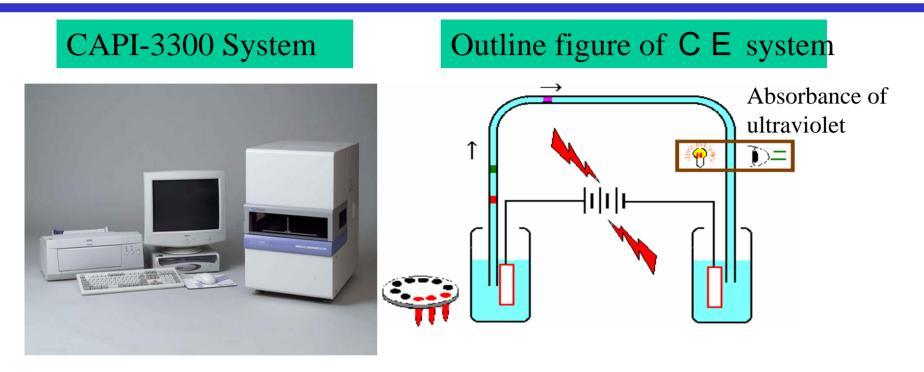
All ingredients in EP acid were measured by capillary electrophoresis (CE) measuring system.
