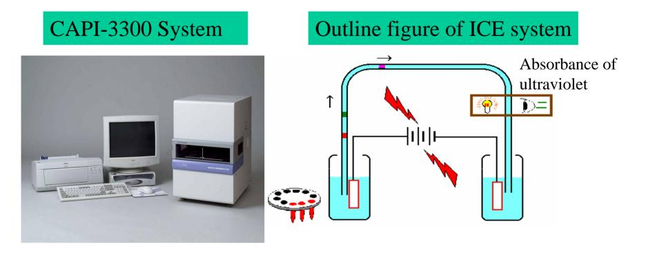
F<sup>-</sup> and SO<sub>4</sub><sup>2-</sup> in EP acid were measured by Ion Capillary Electrophoresis (ICE) measurement system.
