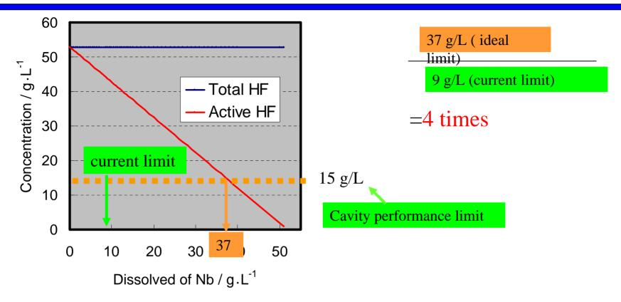
If we could eliminate the evaporation of active 【HF】, we can use EP acid 4 times more efficiently. In other words, the cost of EP acid in mass-production become 1/4.
