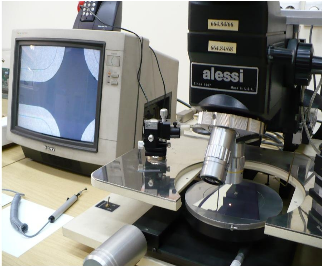
Alessi probe station used for visual inspection of Hamamatsu detectors
