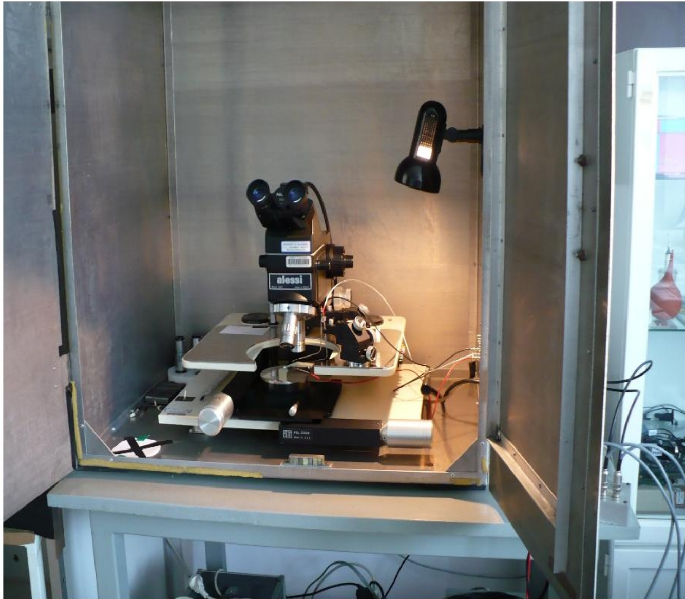
Alessi probe station used for electrical measurements on Hamamatsu detectors
