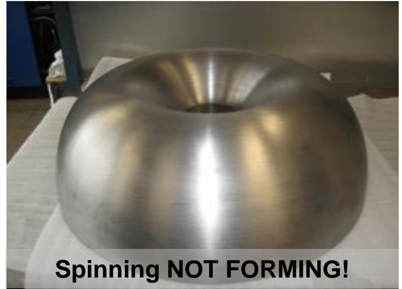
FNAL SSR1 End-Wall Formed From a single Nb Sheet
