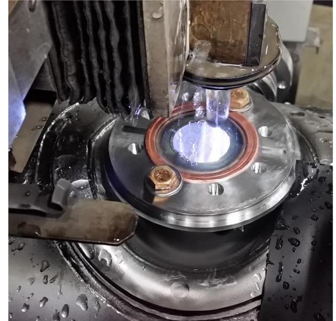
Beam Aperture Wire-EDM
