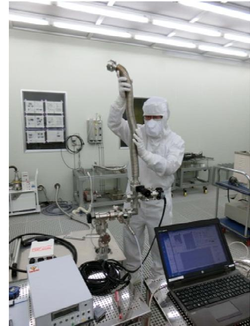
After hitting the bellows, we saw the particle count. Particle exists even though we blow inside the bellows by the ion gun.
