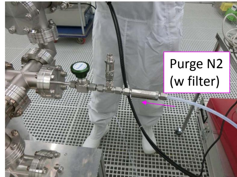
Anyway, we saw the particle count during N2 purging both with and without filter of 5L/min flow
