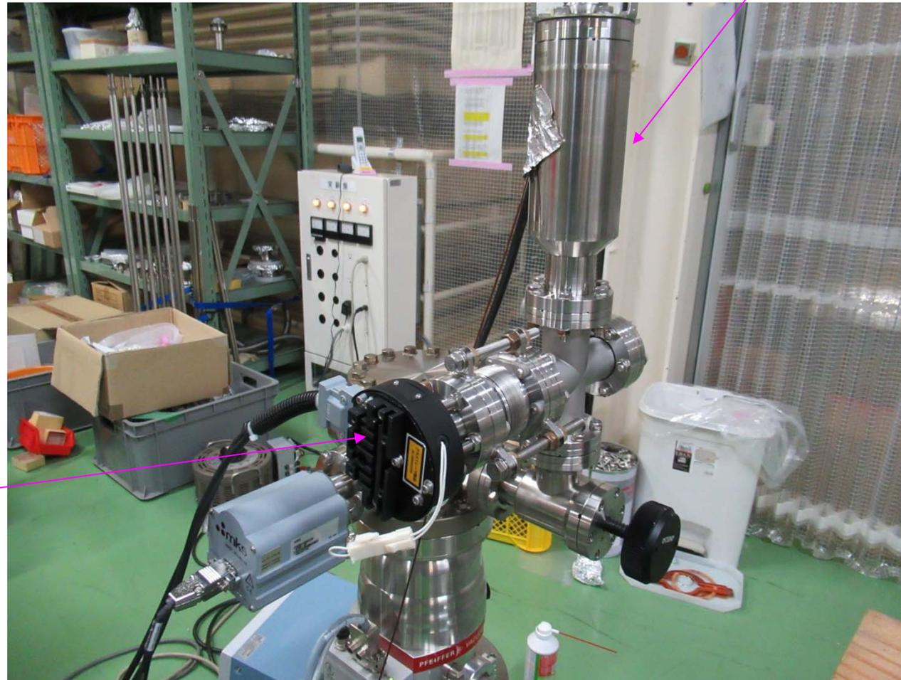
Now under testing of new NEG pump of ZAO with a vacuum particle sensor
