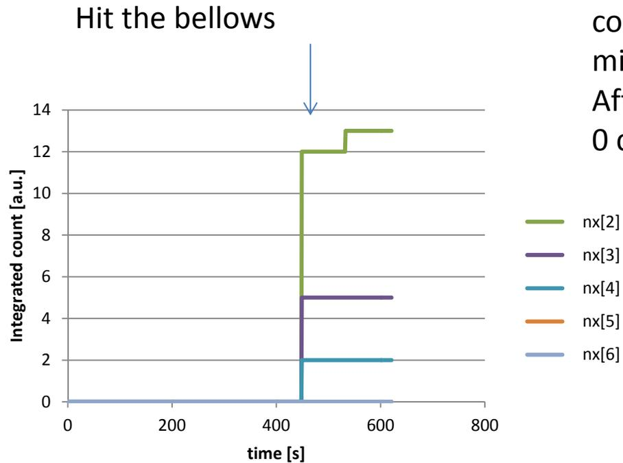
Bellows was connected after 10 min. ion gun blowing. After blowing, we saw 0 count in the bellows.
