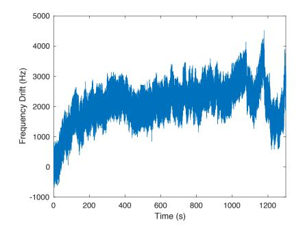
Demonstration of the length stability requirements for ALPS II with a high finesse 10 m cavity
