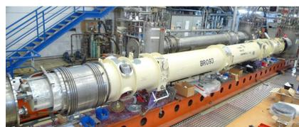
HERA dipole on the magnet test bench
