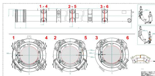
Figure 1: schematic view of a modified HERA dipole
