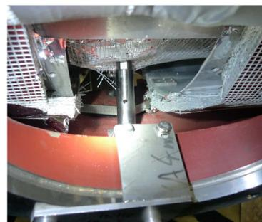
Figure 6: the pressure prop installed at position 5, after straightening
