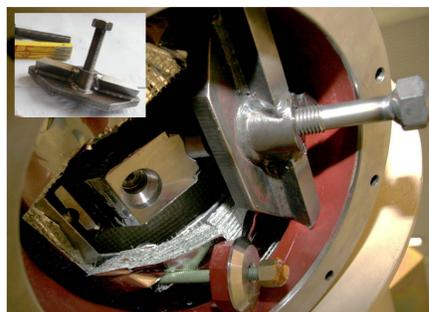
Figure 5: the 'pressure screw' installed at position 5
