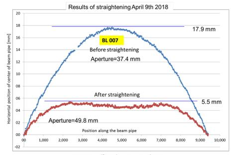
Figure 7: comparison of the beam axis position before and after straightening
