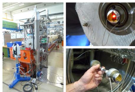
Figure 4: survey of the cold mass position before straightening (left, laser tracker - right, the 'mouse')
