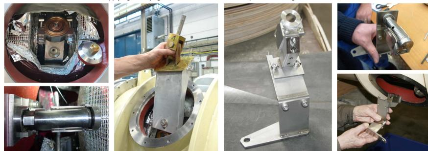
Figure 2: different phases of the pressure prop installation at pos. 1 and 3
