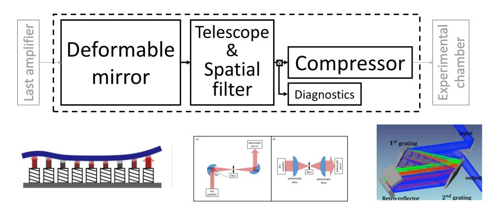
Different grating technologies under evaluation to address main issues with higher repetition rate. Strategy includes **reduction** of the thermal load at high average power, **cooling** of residual heat and **control** of thermal effects on compression quality.
