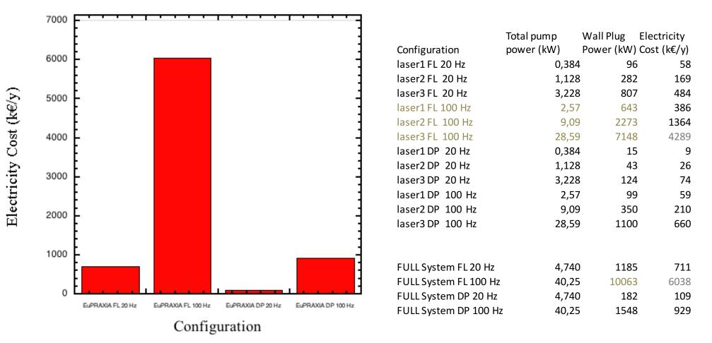
Reduction of electricity running costs due to higher diode efficiency
