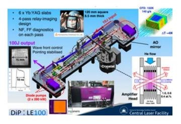
DIPOLE<sup>(1)</sup> 100 @ CLF-STFC DPSSL Yb:YAG, cryogenic He cooling 100 J @ 10 Hz, @515 nm Planned developments: 10J @ 100 Hz
