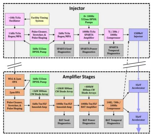
Laser system designed to deliver 7J/30fs/230TW at 100Hz: average power of this system = 700W
