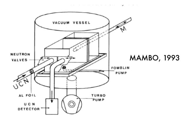
Neutron lifetime determined by measuring number of **neutrons** at beginning and end of experiment
