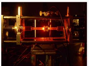
When the ring is rotating, the difference in optical path in the two direction is translated in a frequency difference:
