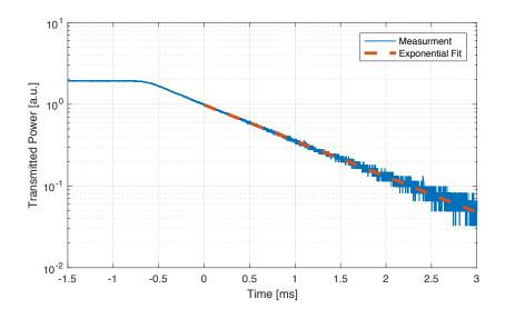
Demonstration of the length stability requirements for ALPS II with a high finesse 10 m cavity
