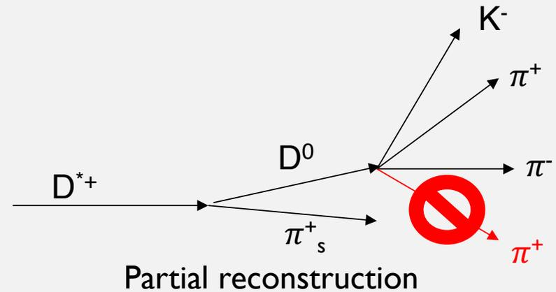
$$\epsilon(\text{track}) = \frac{N_{\text{full}}(D^* \rightarrow D^0(\rightarrow K\pi\pi\pi)\pi_s)}{N_{\text{part}}(D^{*+} \rightarrow D^0(K\pi\pi[\pi])\pi_s^+)}$$
