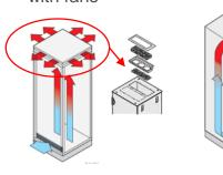
Additional bypasses for air flow necessary are reducing the efficiency
