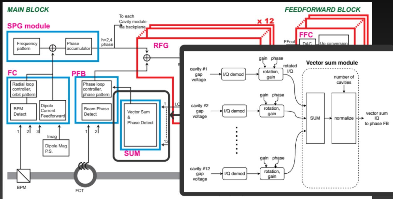
(Blue) common functions for whole system / (Red) for each of 12 cavities
