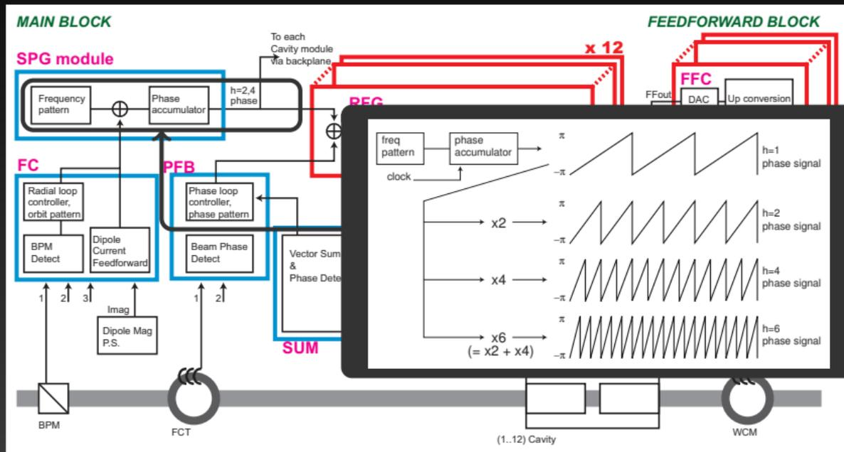
(Blue) common functions for whole system / (Red) for each of 12 cavities
