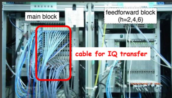
Existing system uses cables and parallel backplane.
