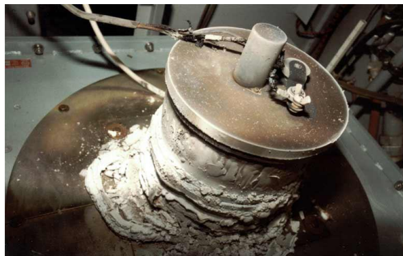
Klystron melt-down after arc, TV transmitter
