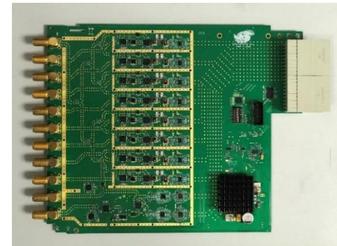
• 8-channel downconverter with 1-channel VM
