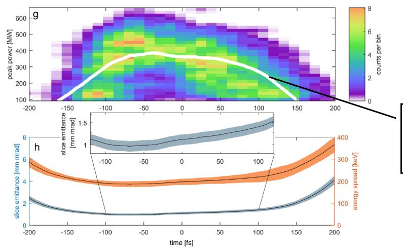
Measured emittance and current profiles and Ming Xie formalism very nicely model lasing in different regions of electron bunch
