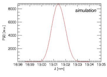
Seeding transforms the FEL into a fully coherent light source
