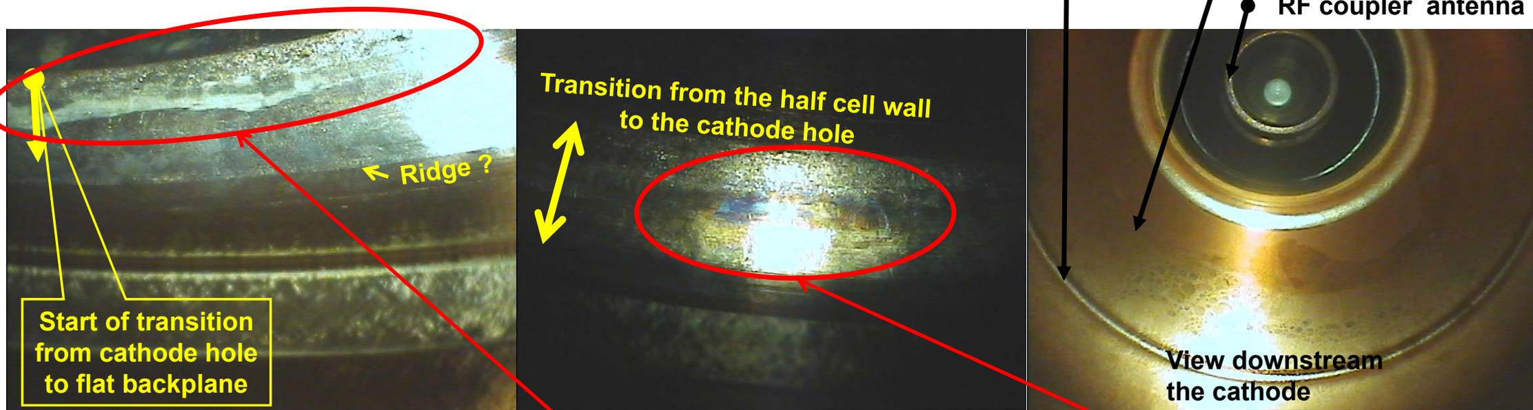
White (calcareous-like) traces and color changes (like from high temperature gradient or from burning) was observed on the rounding between cathode hole and flat backplane
