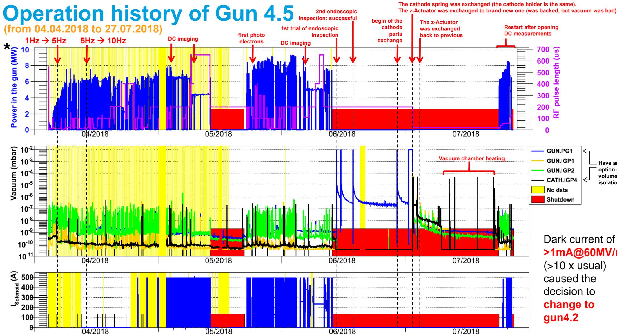
\* The power readings are presented from 10MW dir. coupler. The readings are not 100% reliable.
