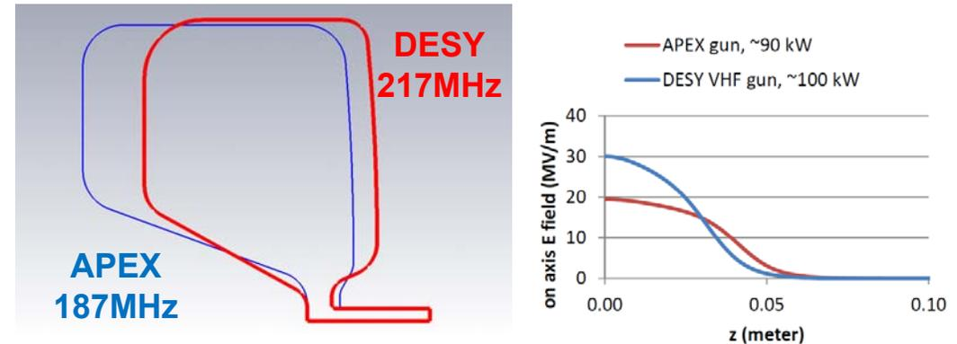
Preliminary injector simulation with DESY VHF gun (100 pC)
