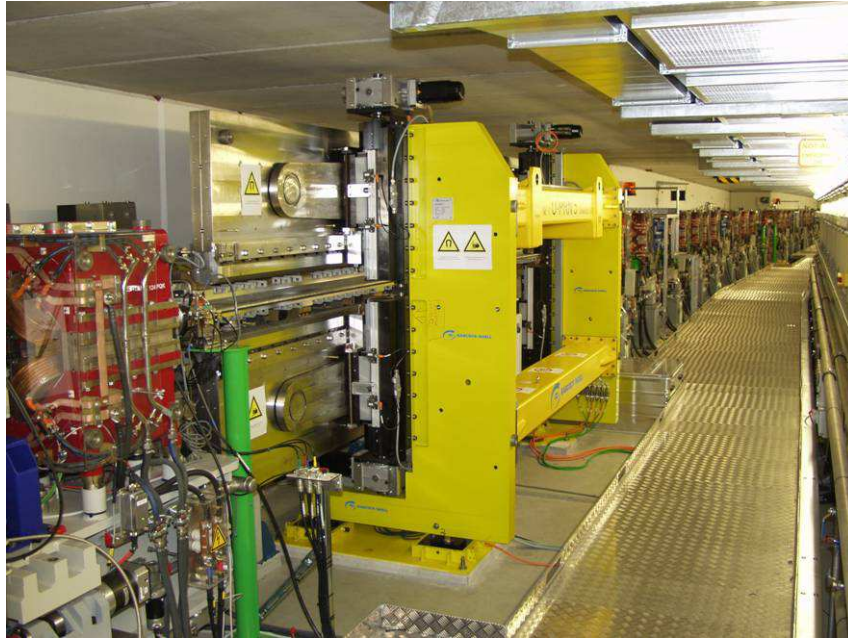
very flat undulator vacuum chambers
