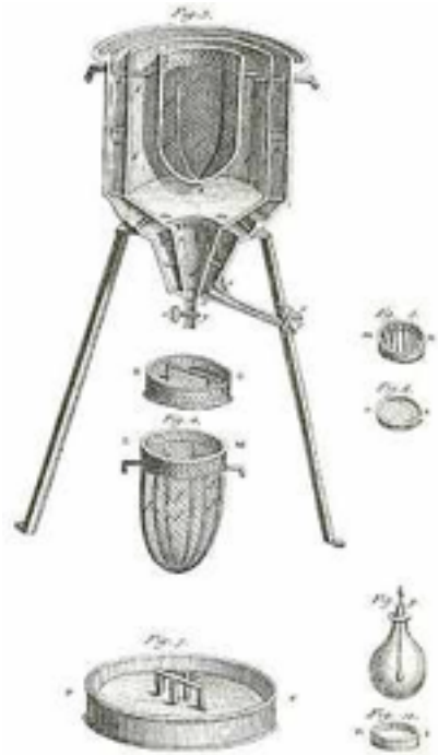
Ice-calorimeter from Antoine Lavoisier's 1789 Elements of Chemistry .
