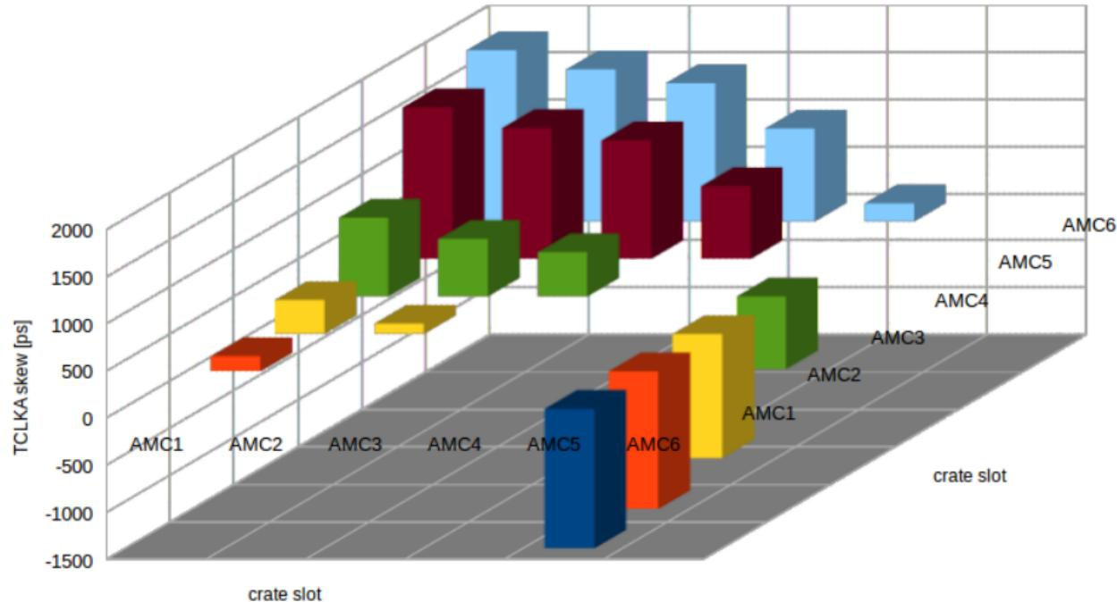
Clock skew can be removed on AMC board in FPGA with built-in PLL (Phase-Locked Loop) or DCM (Digital Clock Manager)
