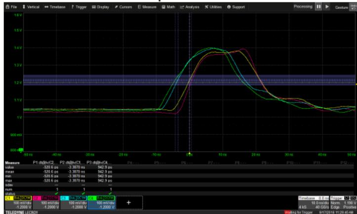
after - clock phase tuned to the specific slot
