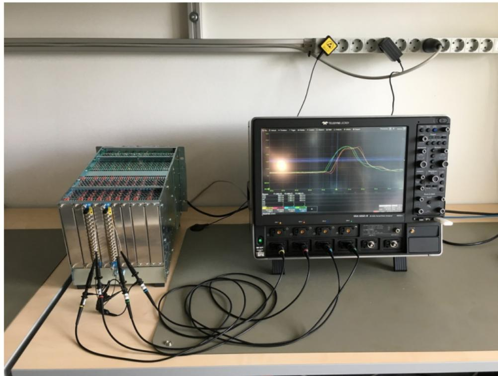
Measurements of clock (TCLKA) skew (in ps) between different slots in MTCA crate:
