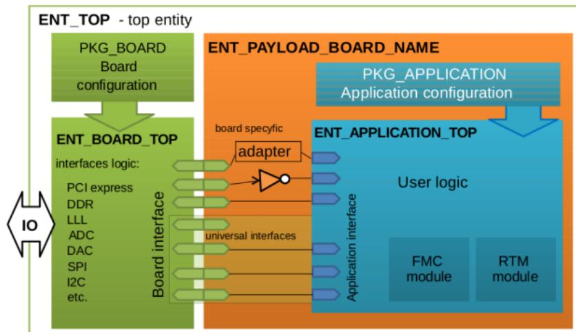
Figure 2: VHDL code block structure
