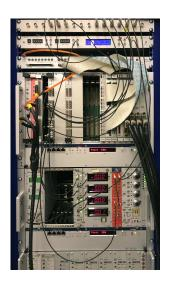
Mostly VME or NIM modules: Counter, Timer, GPIO, ADC, DAC, HV supplies, filter amplifiers, discriminators and lots of motor controllers
