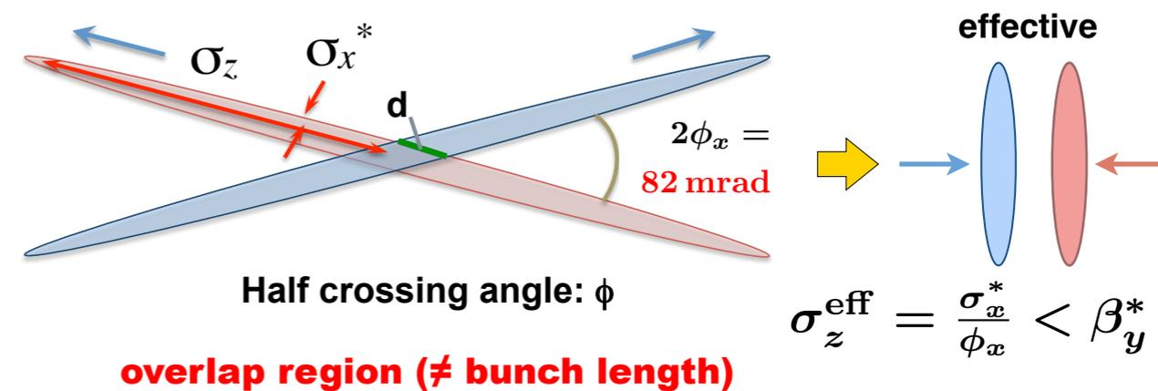
Strong focusing of beams down to vertical size of  $\sim 50\text{nm}$  requires **low emittance beams** and **large crossing angle**  $\Rightarrow$
