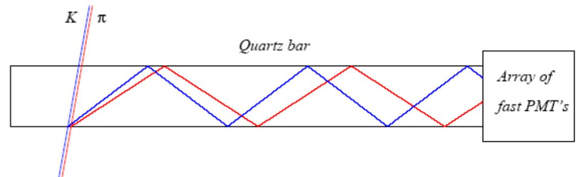
$\theta_c$  is reconstructed from hit position (x,y) in the PMT and from time of propagation
