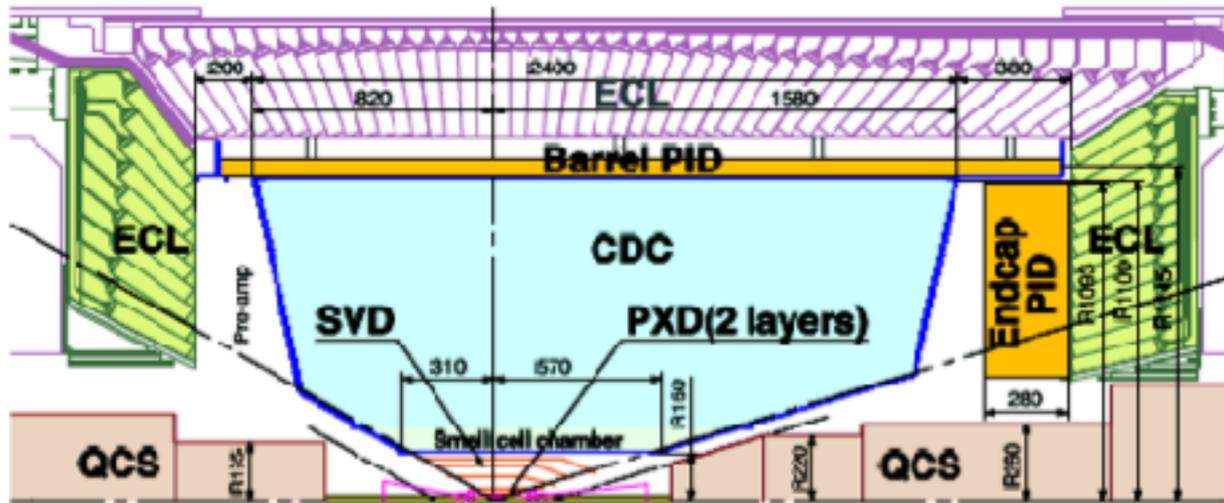
Belle calorimeter: 8736 CsI(Tl) crystals
