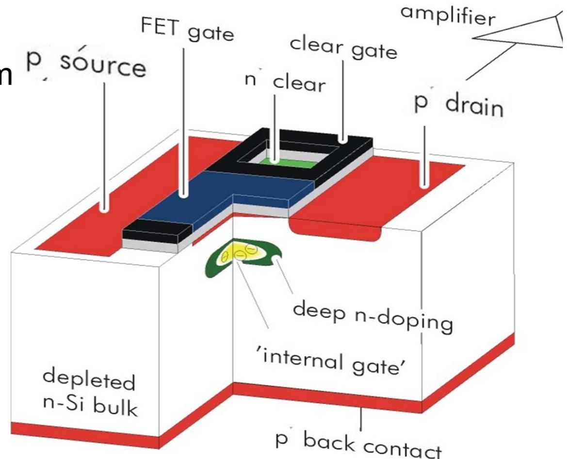
Transistor on only during readout:
