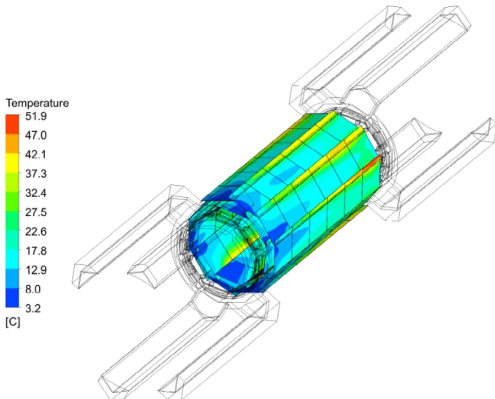
Example CFD simulation result for vertex detector.
