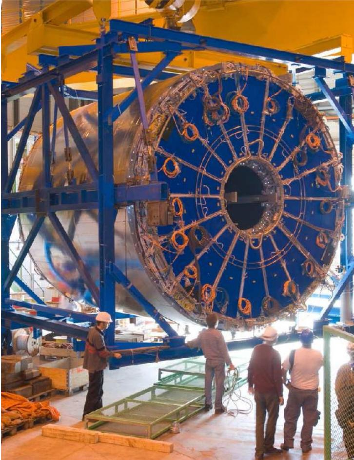
The chamber was designed to study the heavy ion collisions at the LHC (Pb with 2.7 TeV/nucleon  $\rightarrow \sqrt{s} = 574$  TeV ).
