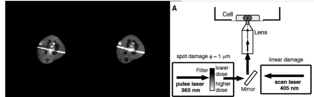
(a) 20 sec after irradiation (b) 200 sec (c) Irradiation and scanning system
