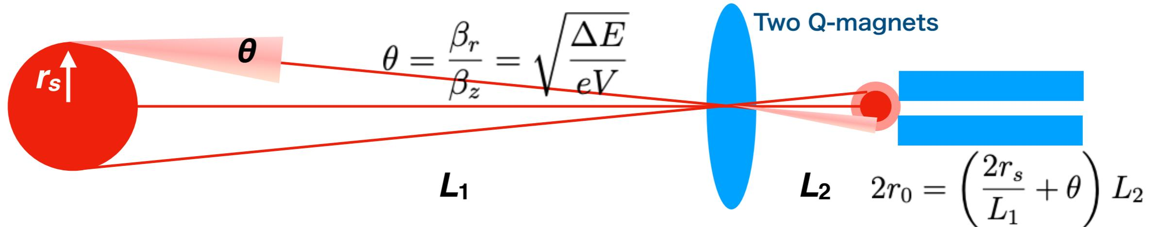
The cross section of the e-beam at the DLA entrance is a function of the source size  $r_s$  and the beam divergence angle  $\theta$ .
