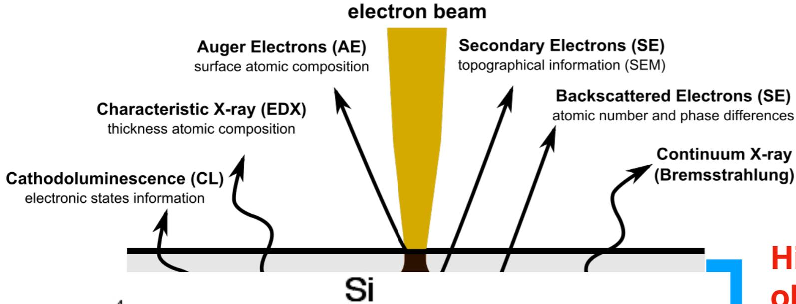
**High-energy electron enables to observe the depth of 3D LSI.**
