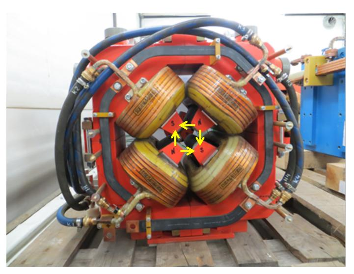
Is this quadrupole focusing or defocusing in the horizontal plane?
