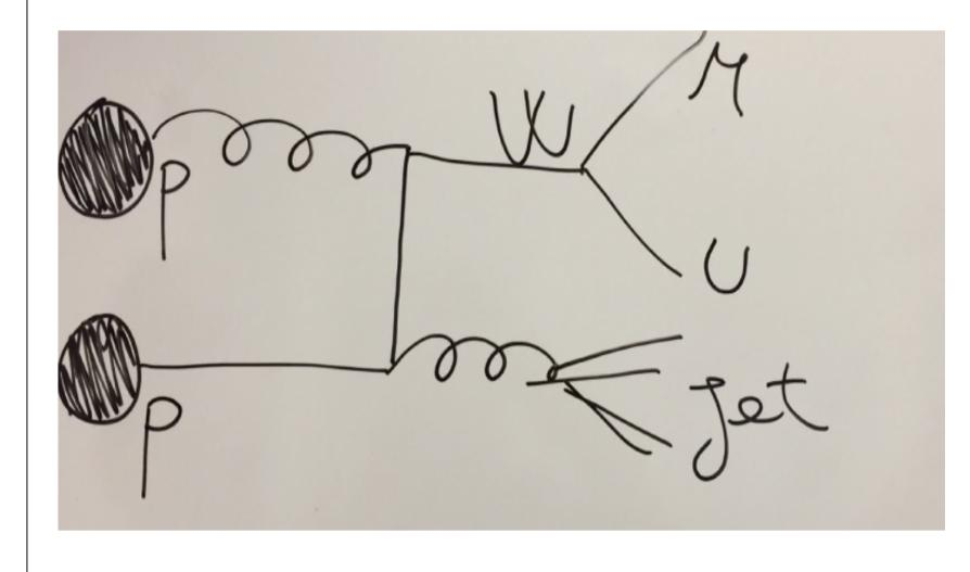
Herewe have two protons, colliding, produce a W boson, which decays in a muon and neutrinos, and jets. So, at the final stage this may seem the decaying of an Higgs boson, while it isn't actually.
