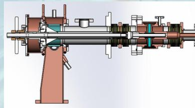
XFEL/ILC/LCLS-II or other type **variable power coupler.** Peak power 30 kW, average 4 kW,  $Q_{\text{ext}} 1E7-5E7$ , two windows.
