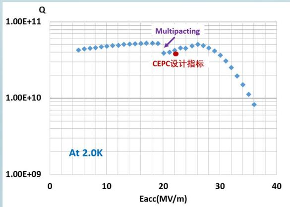
After N-doping,  $Q_0$  increased obviously at low field for both 650MHz 1-cell cavities.
