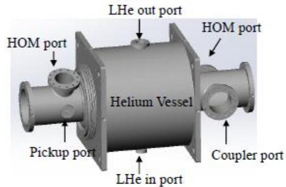
650 MHz 2-cell cavity + Helium Vessel 3D module
