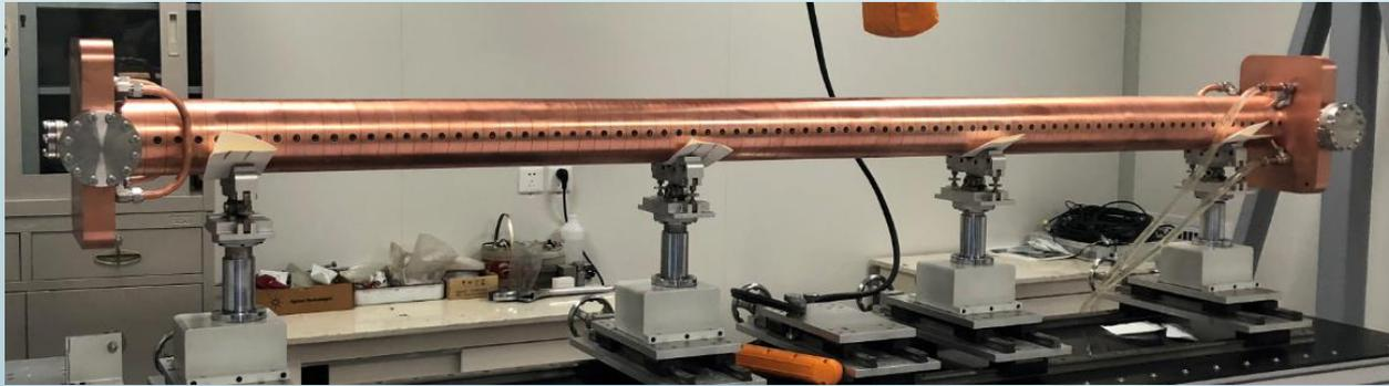
Accelerating structure under cold test
