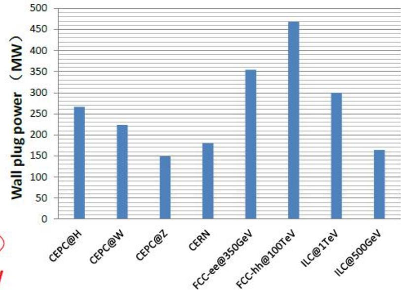
CEPC TDR stage to reduce power consumption less than 266MW by green design
