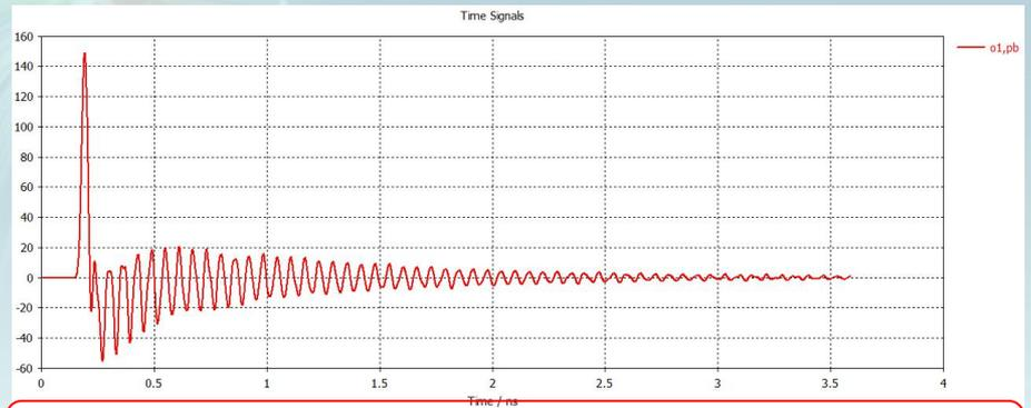
Due to the short bunch length, signal has many resonance hump, signal amplitude proportional to the bunch charge.
