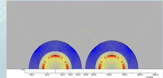
There is iron yoke around the quadrupole coil for QF1. Since the distance between the two apertures is larger enough and there is iron yoke, the field cross talk between two apertures of QF1 can be eliminated.
