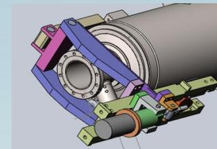
XFEL/LCLS-II type **end lever tuner.** Reliability. Large stiffness. Piezos abundance, radiation, overheating. Access ports for easy maintenance.
