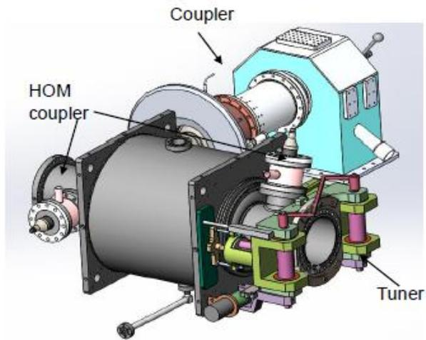
Cavity + Coupler + HOM Coupler + Tuner
