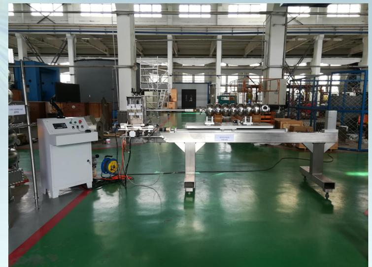
Cavity inner surface repairing system
