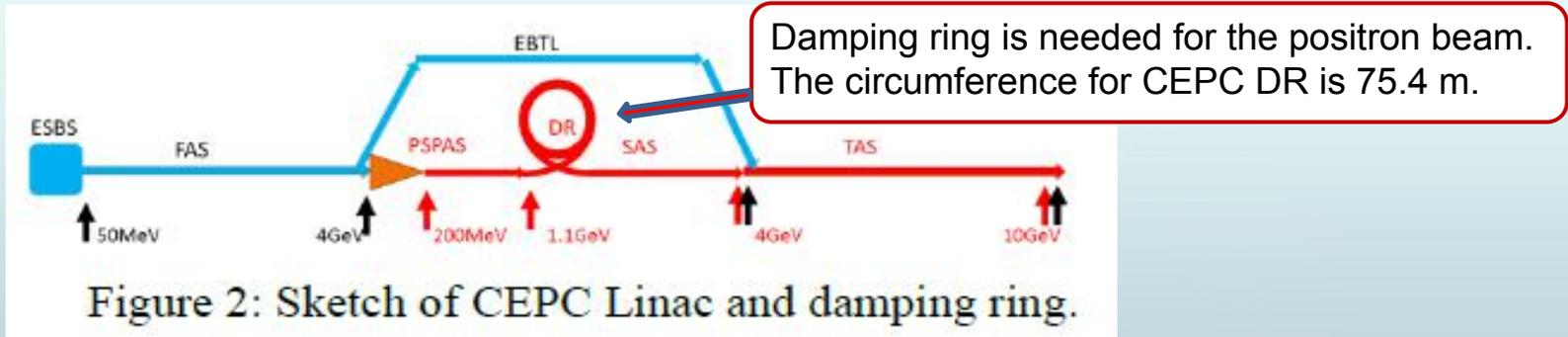
The injection beam structure of CEPC Linac is pulsed operation.
