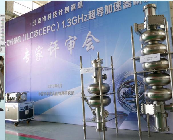
CEPC 650MHz 2cell and 5 cell cavities
