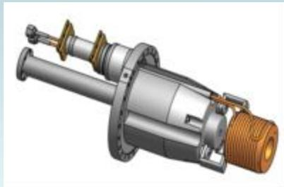
The mechanical design of FLUX concentrator
