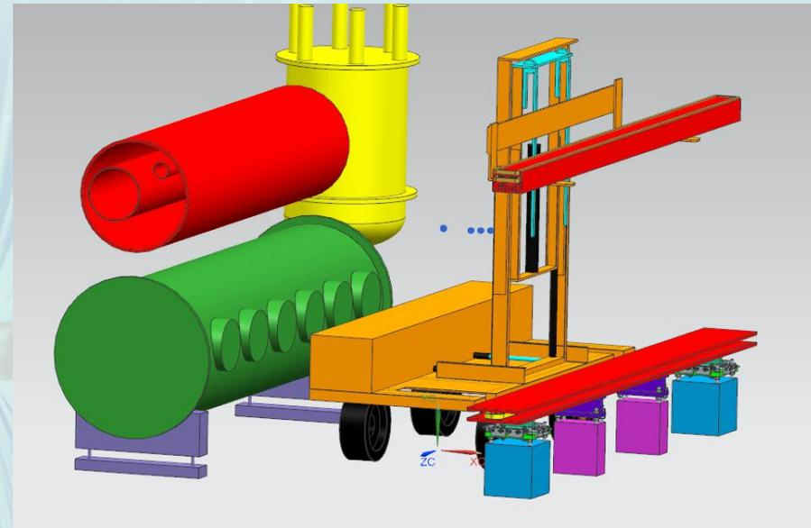
Schematic of transport vehicle of magnets
