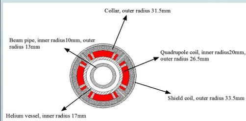
Room-temperature vacuum chamber with a clearance gap of 4 mm
