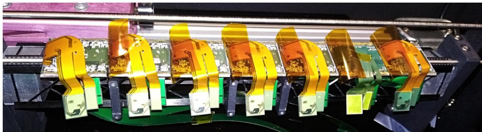
Electrical outer barrel prototype with 7 FE-I4 quads
