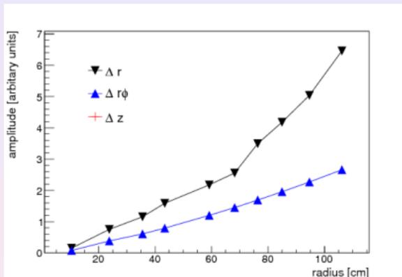
Left: Fit of deformation from eigenvector (5th layer) to second mode.
