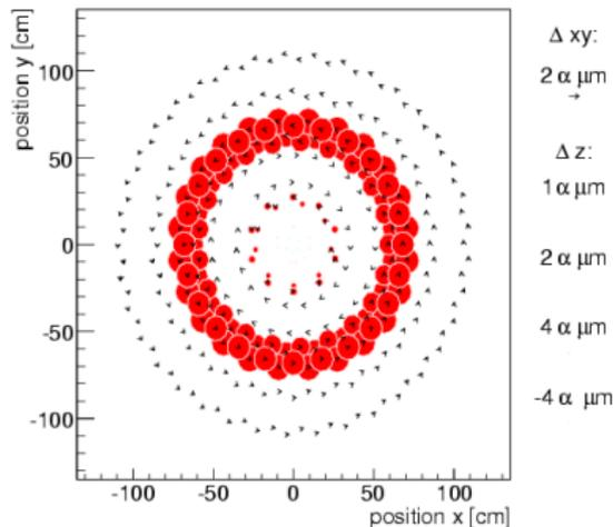
Left: Twist (red: barrel-, black: barrel +), Right: z shearing.
