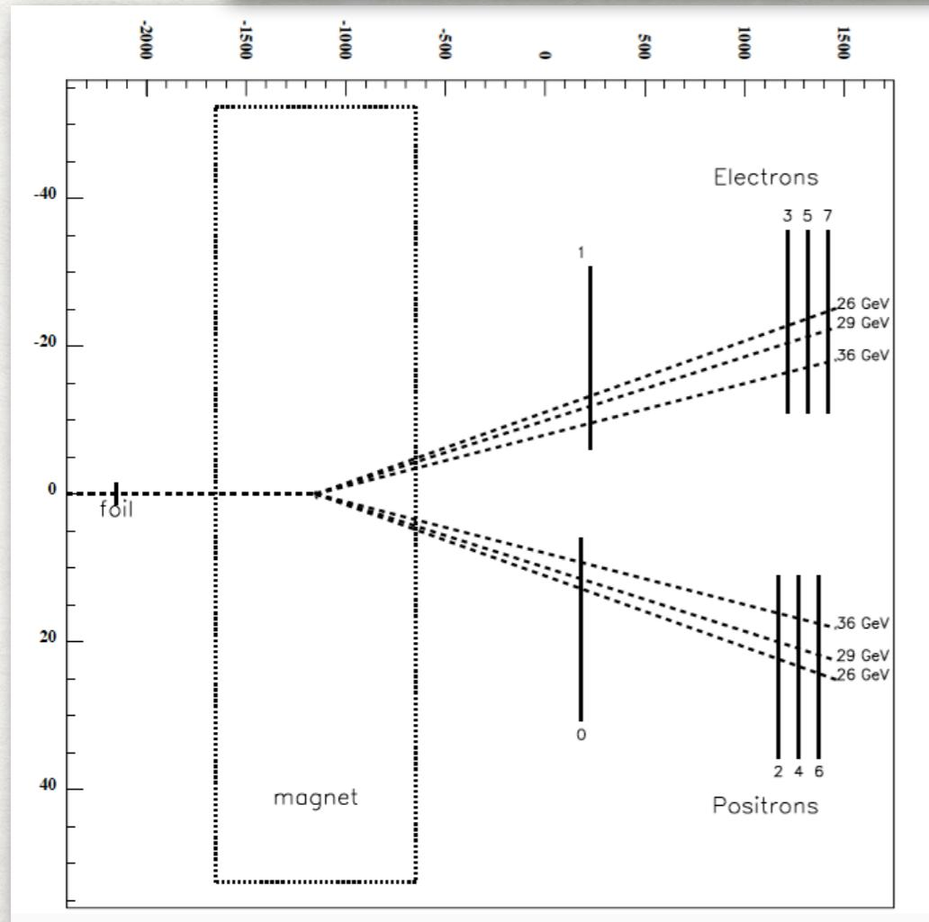
In E144 the data in the two arms of the spectrometer were analyzed independently, and then combined the reconstructed single-particle momentum spectra for comparison to a model spectrum calculated by convolving the simulated photon spectrum with the Bethe-Heitler pair spectrum
