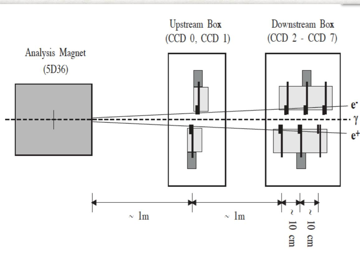
e-/e+ tracks were reconstructed using the 3 back planes of CCD's. All triplets of points from the back CCD planes of a given arm were tested to see if they fit a line intercepting a region near the center of the spectrometer magnet. This set of candidate tracks included many "fake" tracks from thermal noise, and combinatoric background of points from different particles.
