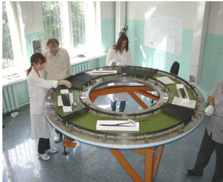
Installation of straws (tests leak tightness)
