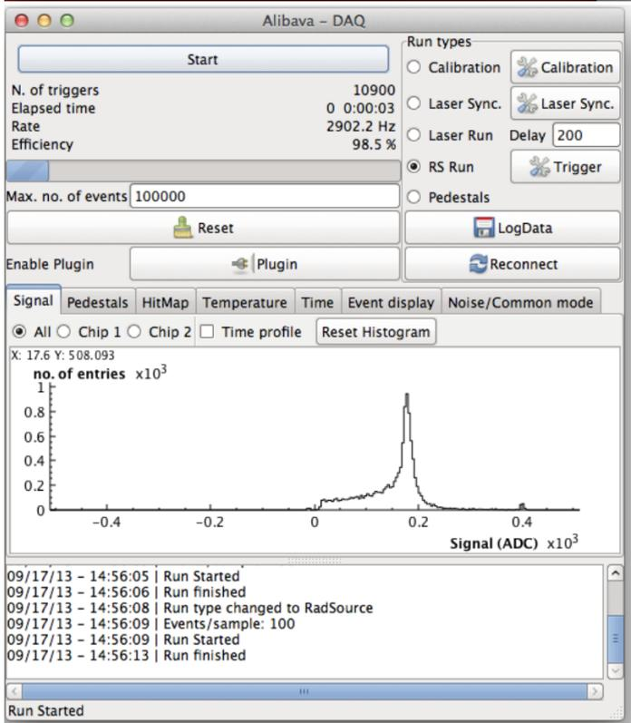
Figure 7: Screenshots of the Alibava GUI. Right Main menu with the full signal, left the time profile.
