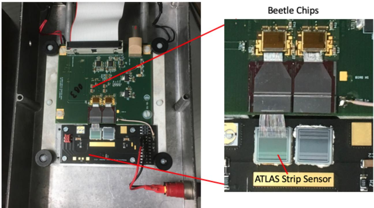
**Figure 4:** Top view of the EDIT2020 Landau setup inside the closed setup box with a zoom-in onto the daughterboard housing the beetle chip and the ATLAS strip mini sensor.
