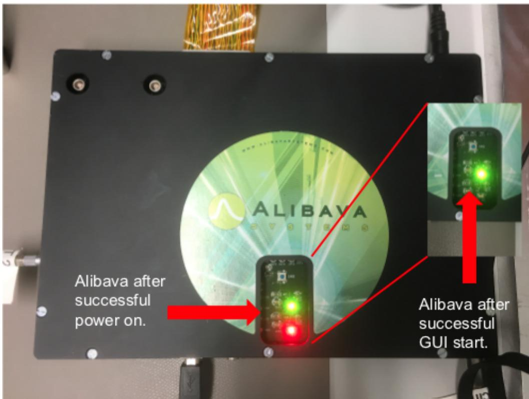
**Figure 5:** Top view of the box housing the Alibava motherboard with the initialization lights.
