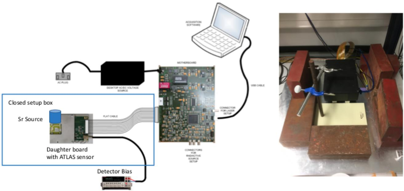
**Figure 3:** Schematic of the laboratory setup for measuring charge deposition (left) and a look inside the closed setup box (right).
