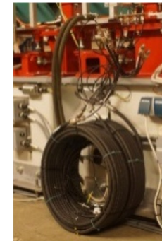
Delayline = 100ns RF cable 1/2" ~26m
