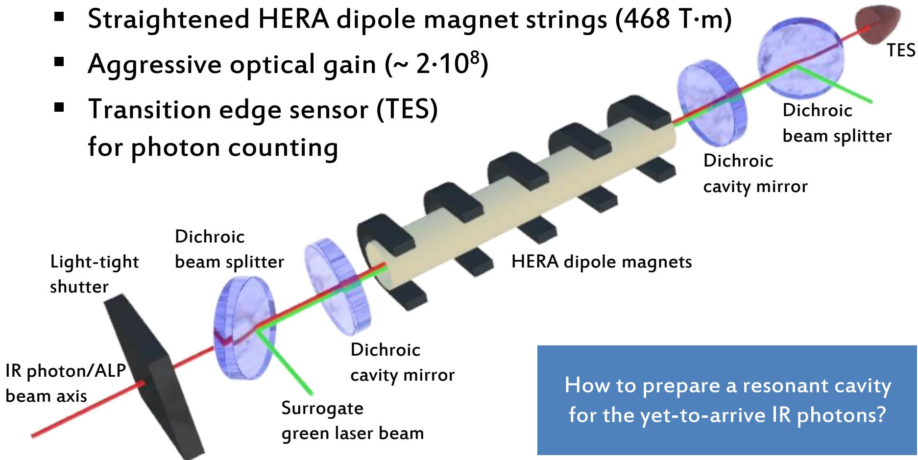
How to prepare a resonant cavity
