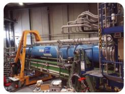
microwave filter-like structure composed of five coupled cavities connected by rectangular irises to increase V
