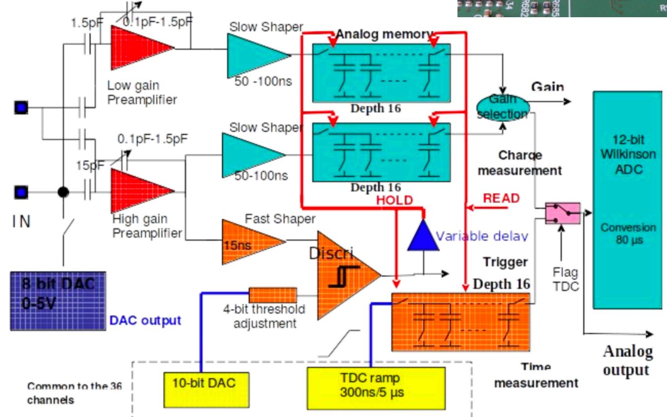
Readout schematic for one channel
