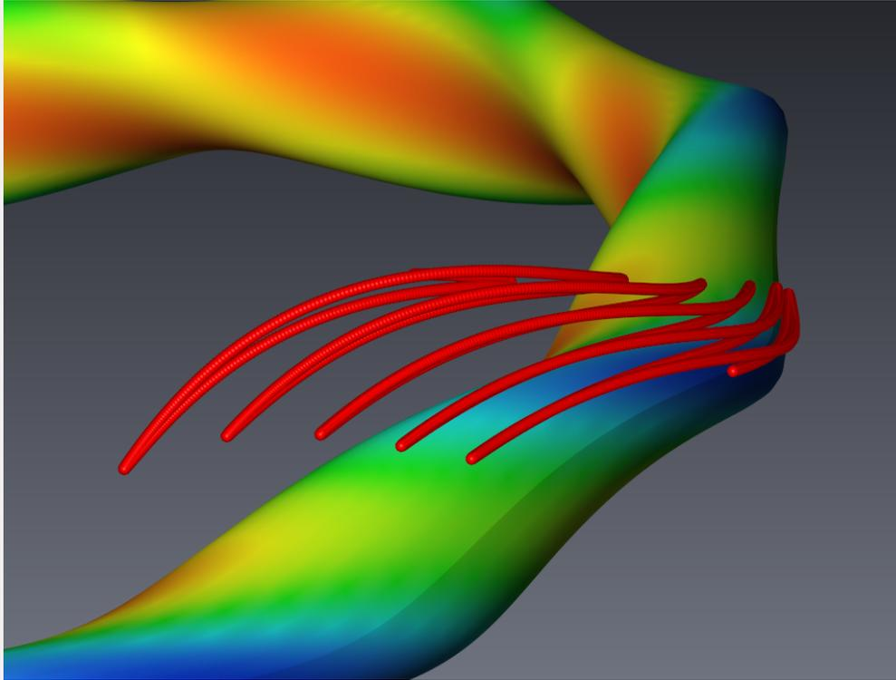
Trajectory of a particle trapped in the region of low magnetic field.
