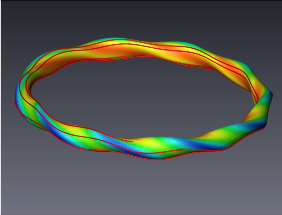
Trajectory of a particle travelling around the torus completely while following a magnetic field line.
