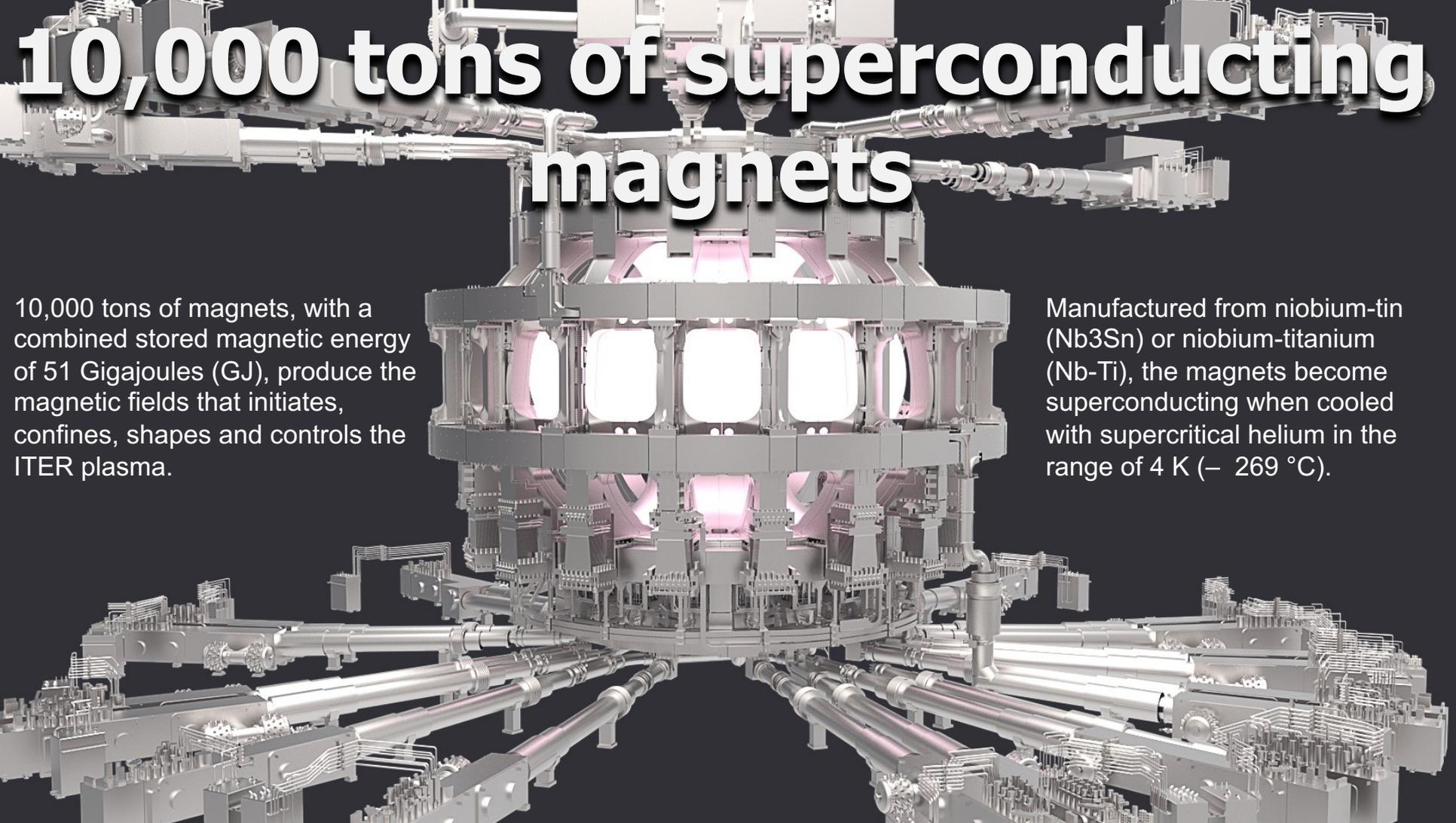
10,000 tons of magnets, with a combined stored magnetic energy of 51 Gigajoules (GJ), produce the magnetic fields that initiates, confines, shapes and controls the ITER plasma.
