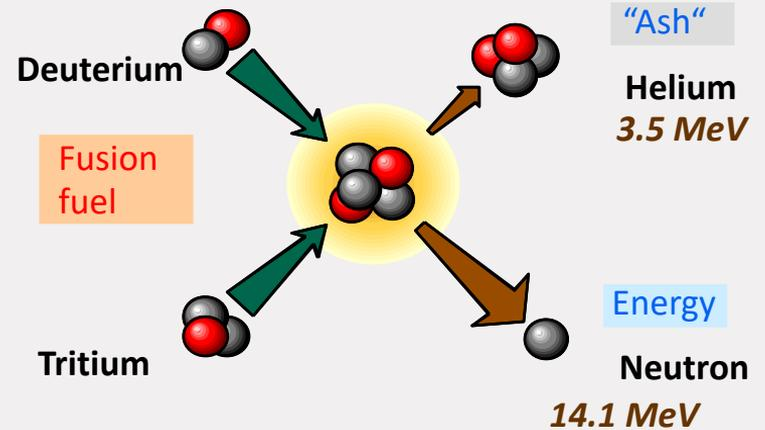
Neutrons from fusion heating up the wall → steam → generator
