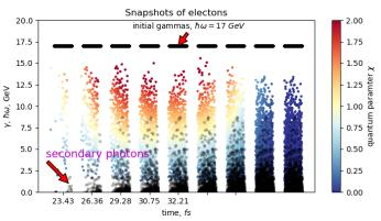
$\gamma$ -bunch generates  $e^{\pm}$  when  $\chi$  is high enough (inside laser pulse) efficiency:  $N_{\gamma}=10^4$  creates  $N_{e^{\pm}}=1092$
