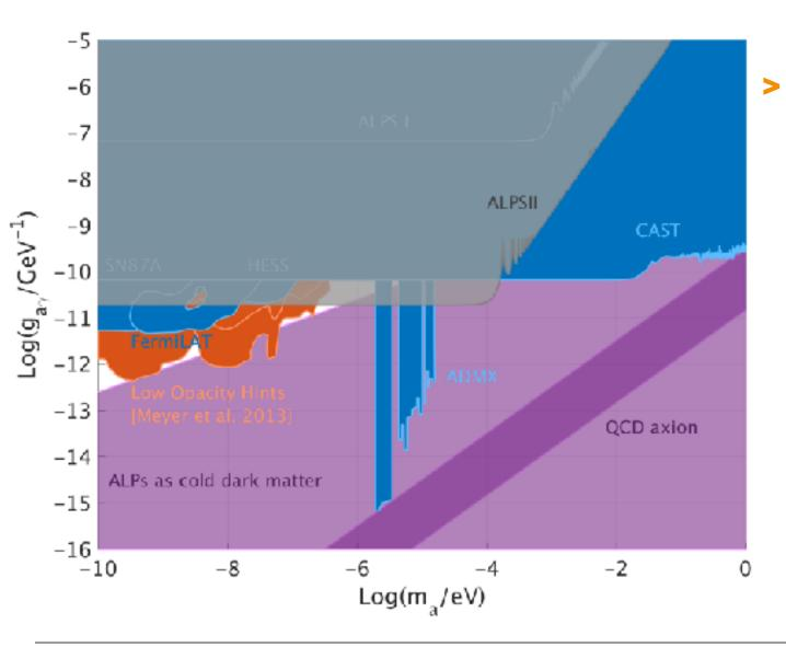
> A sensitivity of experiment for scalar and pseudo-scalar particles with 95 % confidence level at  $g_{ayy}$  = 2 × 10<sup>-11</sup>/GeV for masses below 0.1 meV and an integration time of 20 days.
